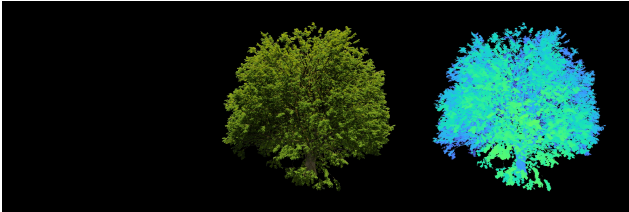
Figure 7. Render output with different settings. Images on the left, middle, and right represents the rendered results of instance annotation, RGB, and depth map, respectively. Instance annotation map was rendered as a very dark images as the pixel values were assigned as one.
